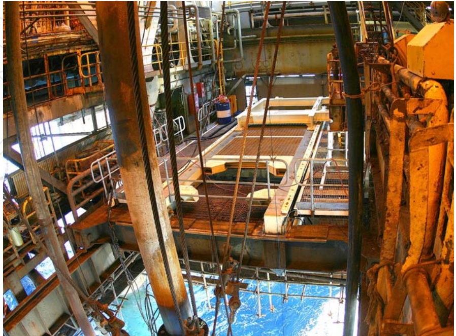
Two stage skidding system as installed in the moon pool area of the Ocean Bounty.
