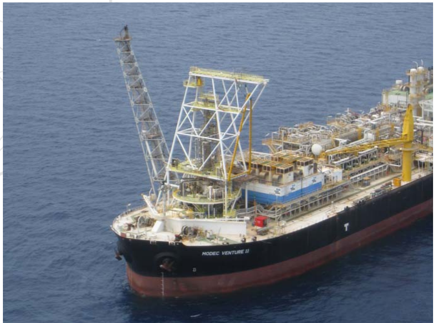
AME's A-frame attached to the MV11's swivel access structure.
