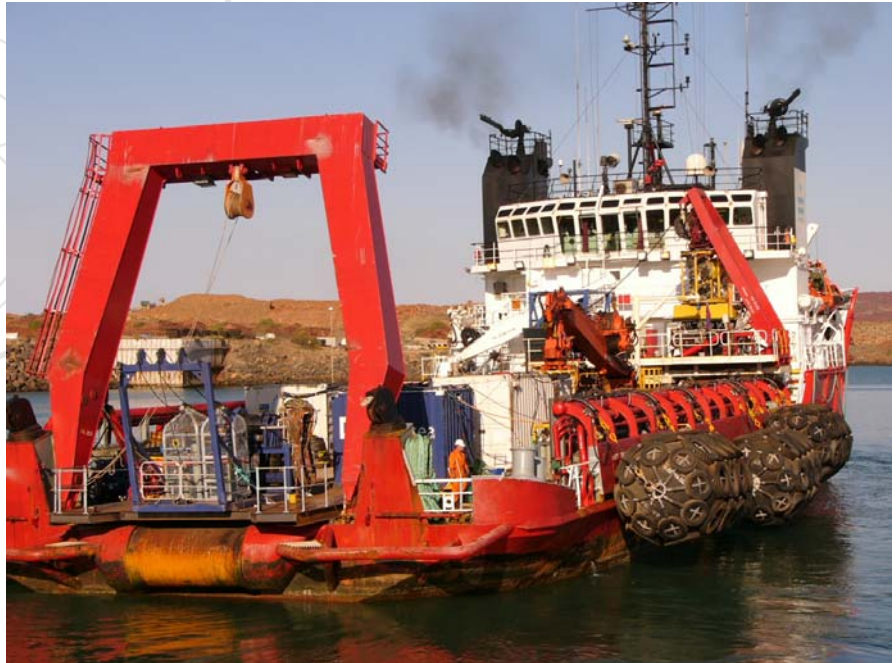
Lady Christine during fender deployment and recovery system testing.
