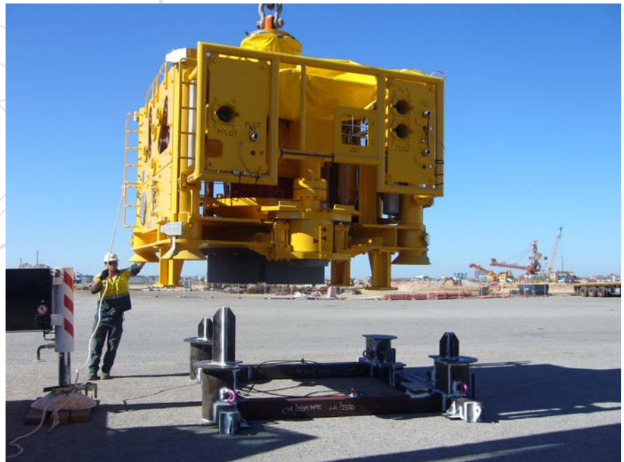
35 tonne Subsea Christmas Tree (XT) being lowered onto transport skid during SIT
